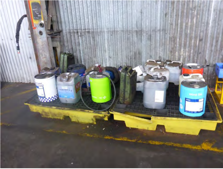
Photo 7 Chemicals stored within bunds
